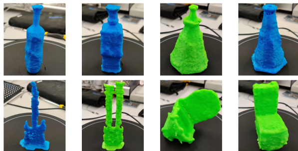
Figure 1: Visualization of the 3D Printed Physical Adversarial Objects Generated by Our Attack Algorithm.
